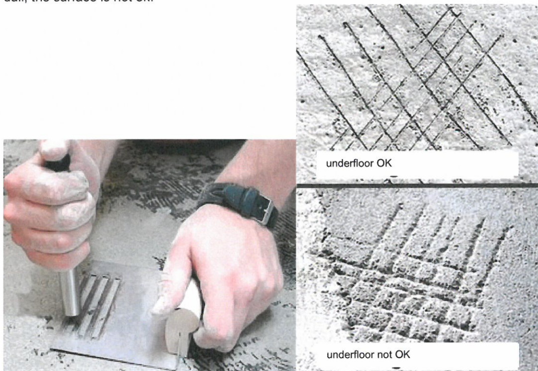
Fig.4. Scratching tool (pen and steel pattern) Fig.5. Scratch test OK (above), not OK (under)
