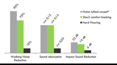
**Conclusion**: The acoustic properties of 2tec2 are far better than hard flooring and within the same range of most textile carpet tiles.
